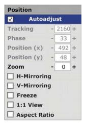
The Position Menu allows picture related adjustments, like manual picture "X" and "Y" positioning (if "Auto center" is set "OFF"), picture mirroring or rotation, etc. Select the menu items by pressing the **[UP]** or **[DOWN]** buttons, uses the **[RIGHT]** and **[LEFT]** buttons to modify the numerical values of the items. Quit the parameter changes using the **[UP]** or **[DOWN]** buttons, close the Input Menu Window by pressing the **[LEFT]** button.
